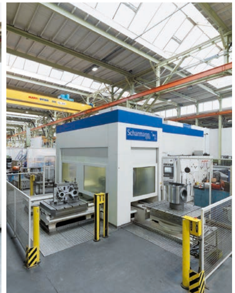
Dörries Scharmann, CNC Boring Mill 4 tables, spindle stroke: 600 mm
