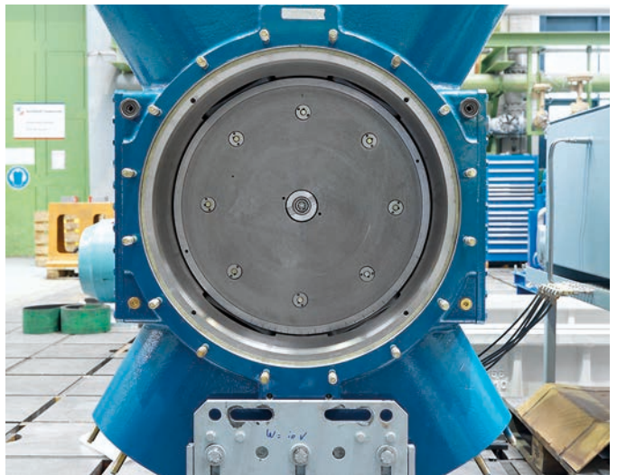
Easy access to piston and cylinder liner
