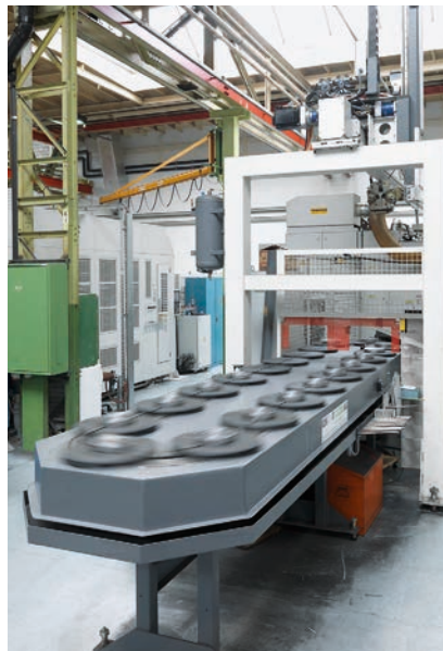
Okuma MacTurn350, Multitasking Center. Fully automatic parts feeding
