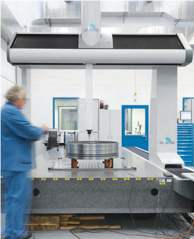
Cutting-edge 3D CNC Measurement Machine for quality inspection
