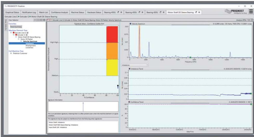
Detection of imbalance failure pattern with trending of the Confidence
