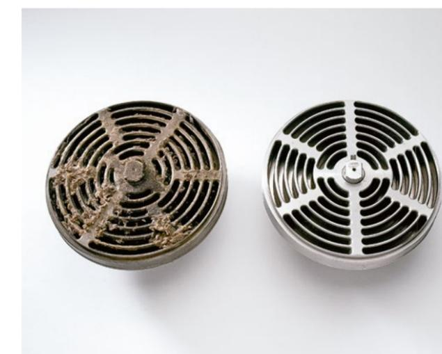
**“After installing the Burckhardt Poppet Valves™ from Burckhardt Compression, our machines have run over 16'000 hours in oxygen service. We are fully satisfied with the results and our maintenance costs have been significantly reduced.”**
